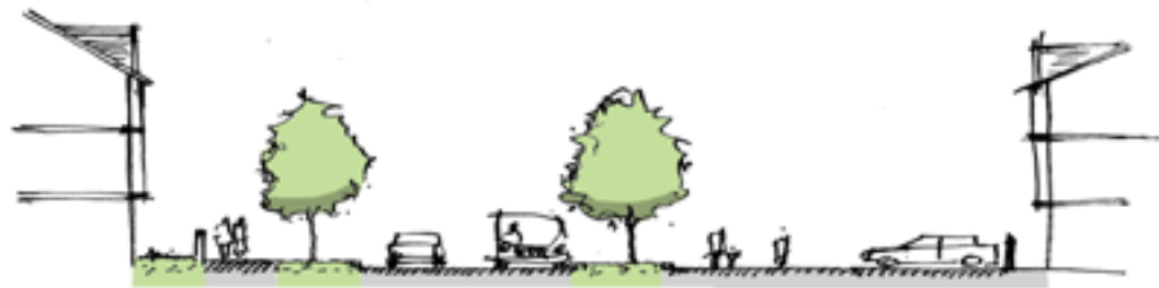
Cross section illustrating how the Pennine Way can be designed to accommodate efficient movement of traffic, whilst providing a high amenity condition for residences along it through the use of a service lane.
