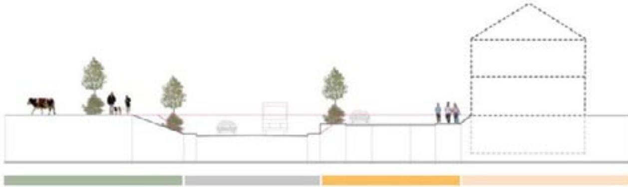
Cross section showing how the Southern Relief Road can manage the interface between road level and building levels, at the same time as providing a high quality and well contained edge to the town.
