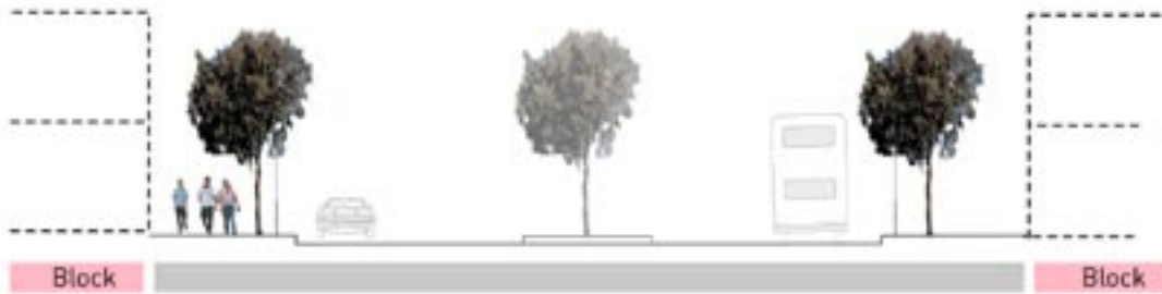
Cross section illustrating how the mainstreet can be designed to accommodate both high link and high place status along its length.
