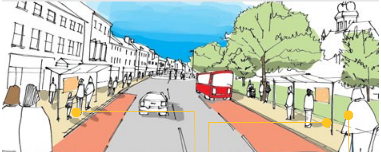
Higher quality public realm, material & furniture Widen footways where possible Provide new local bus node with bus border facilities
