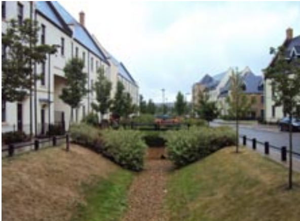
Upton, Northampton is renowned for the integration of sustainable urban drainage into the layout and design of streets.
