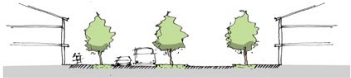
Cross section illustrating how the southern extension mainstreet can be designed to accommodate both high link and high place status along its length through the use of a solid median.
